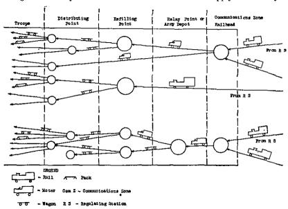
Diagrammatic representation of forward movement of supply in the army.
